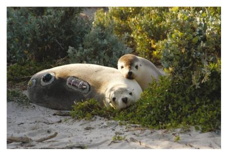
Figure 8 An Australian sea lion, *Neophoca cinerea*, mother and her pup are shown with data loggers attached. The most forward device is a satellite transmitter, the middle device is a time swim-speed and depth recorder, and the last item is a VHF radio.
